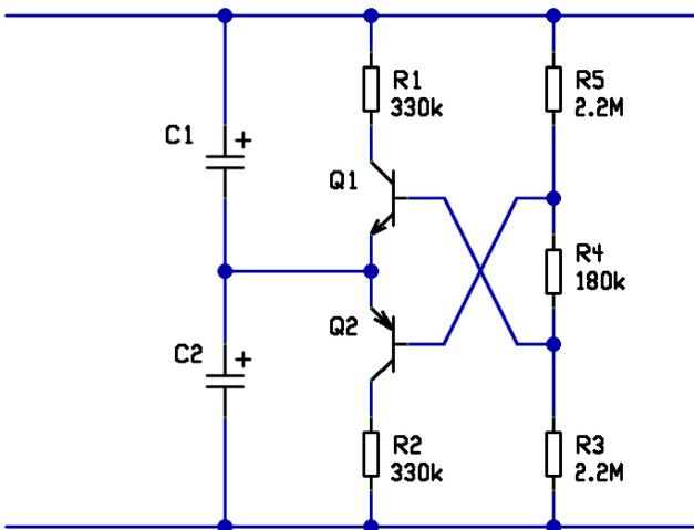
To avoid unnecessary power loss and discharging the pack a suggested C-balance circuit\* can be deployed. It connects equalizing resistors R1 and R2 (by Q1 and Q2 respectively) to the capacitors C1 and C2 only when their voltage difference exceeds certain threshold set by R4, otherwise there is no current flowing and no power loss. As before, R1 and R2 are chosen to dominate leakage current.
