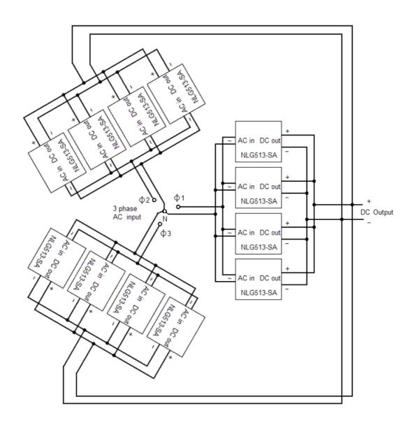
In this particular instance chargers are connected to three phase feed in star configuration, but could as well be connected in delta configuration – this makes no difference in operation.
