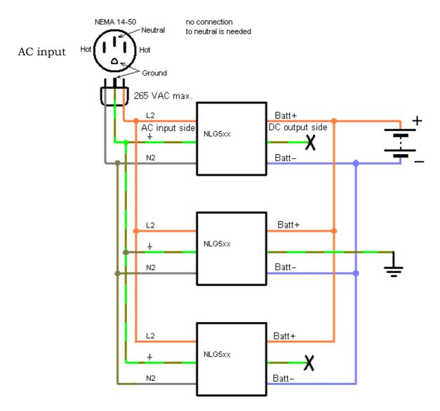
Two or more BRUSA NLG5xx chargers can be connected in parallel to increase total output power thus reducing recharging time. Connection is straight forward and depicted above. As far as chargers concerned, there is no limitation on how many can be paralleled; practical limitations are mains current handling capacity and cost. The array of 12 chargers arranged for 208VAC 3 phase feed is shown on page 2 (example of real life onshore 40kW charging station for an electric boat).
